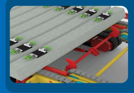
Alignment hooks behind the sleeper pack as it is lowered onto the conveyor tracks.
