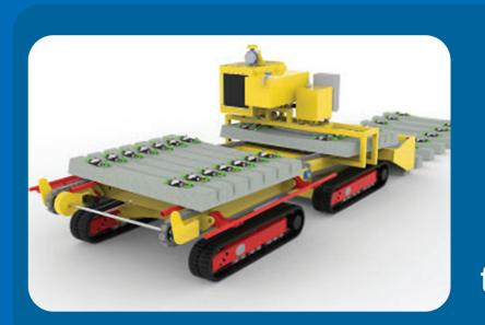
Conveyor tracks move sleepers against the alignment hooks to turn the pack square to the frame of the machine. Bars to the sides of the newly loaded pack can be raised to push the pack across the machine to centre the sleepers.
