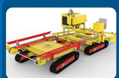
Two round bars between the conveyor tracks of the loading deck can be raised when the deck is empty to protect the conveyor tracks as a pack of sleepers is lowered onto the machine.
